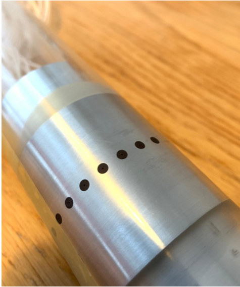
(a) Smooth cylinder - pressure tap close-up.
