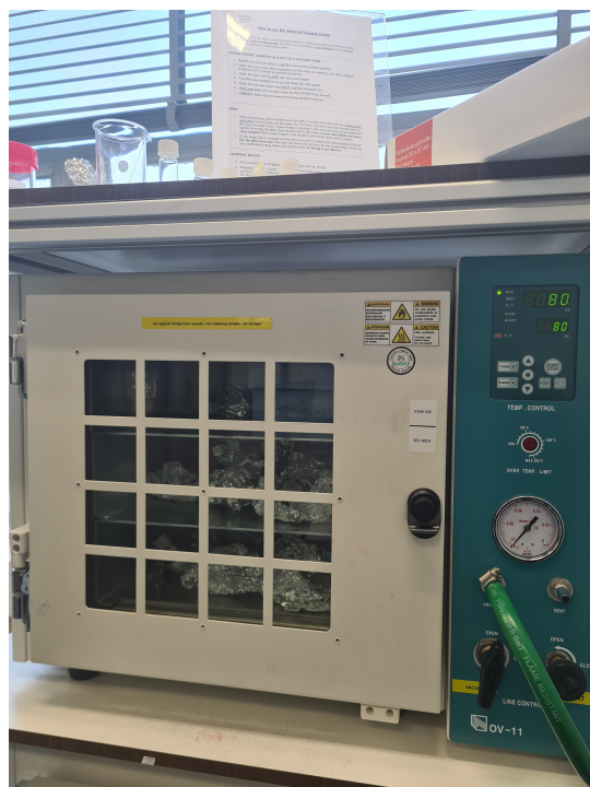
Figure 4.3: Dry vacuum chamber for degassing the components of the batteries.
