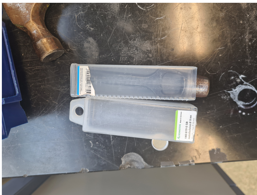
Figure 4.1: Tool for the circular shape of the separator with diameter of 19mm. A similar tool with diameter 12.77mm was used for the LFP cathode electrode.
