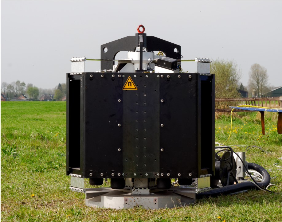
Figure 2.2: Prototype vibrator, based on LSMs, deployed in the field.
