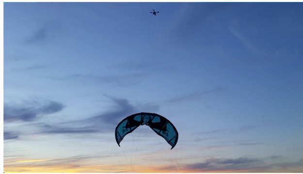
Fig. 1 Custom made drone launching a 9 m 2 kite. Photo credits: Marcos Jerez Venegas.
