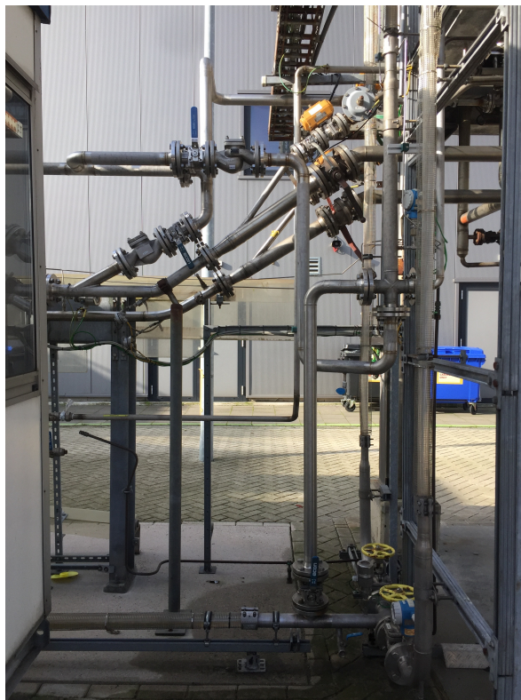
Figure B.10: Side view of the riser base, also showing the injection points of both water and air.
