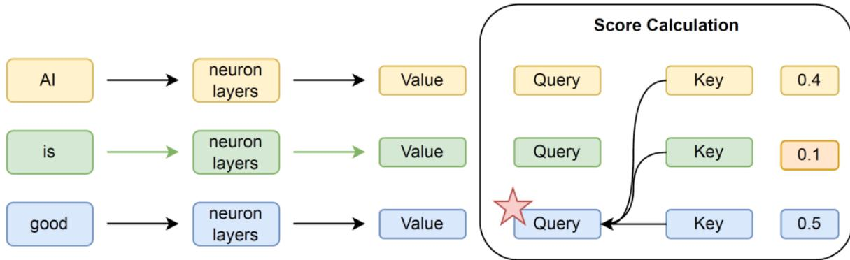
*Illustration of how the word "good" is processed and updated through the self-attention mechanism when the input phrase is "AI is good".*
