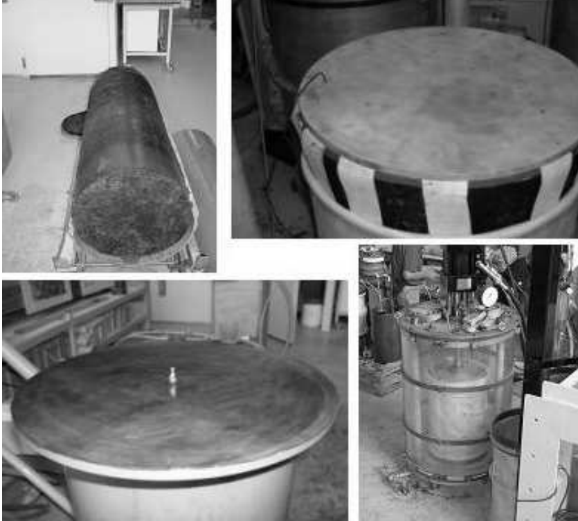
Figure 7.2: a) Sample before trimming b) Drainage strips, top plate and porous stone c) Top plate and pore pressure transducer d) Complete set-up
