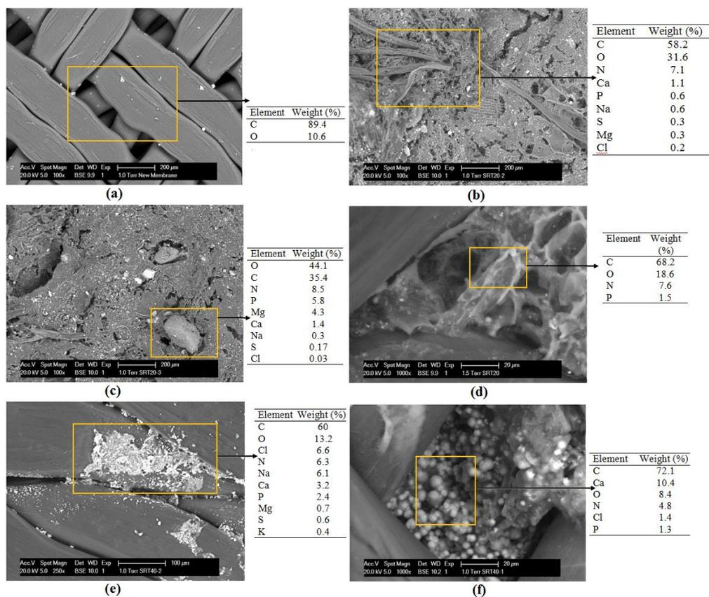
**Figure 5.2.** ESEM images: (a) virgin support material, (b)-(c) DM layer at the end of operation period, (d) EPS-like material, (e) partial gel layer under the DM layer, (f) spherical structures formed under the DM layer.
