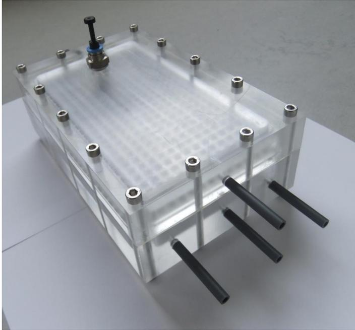
**Figure 6.2.** External membrane module.
