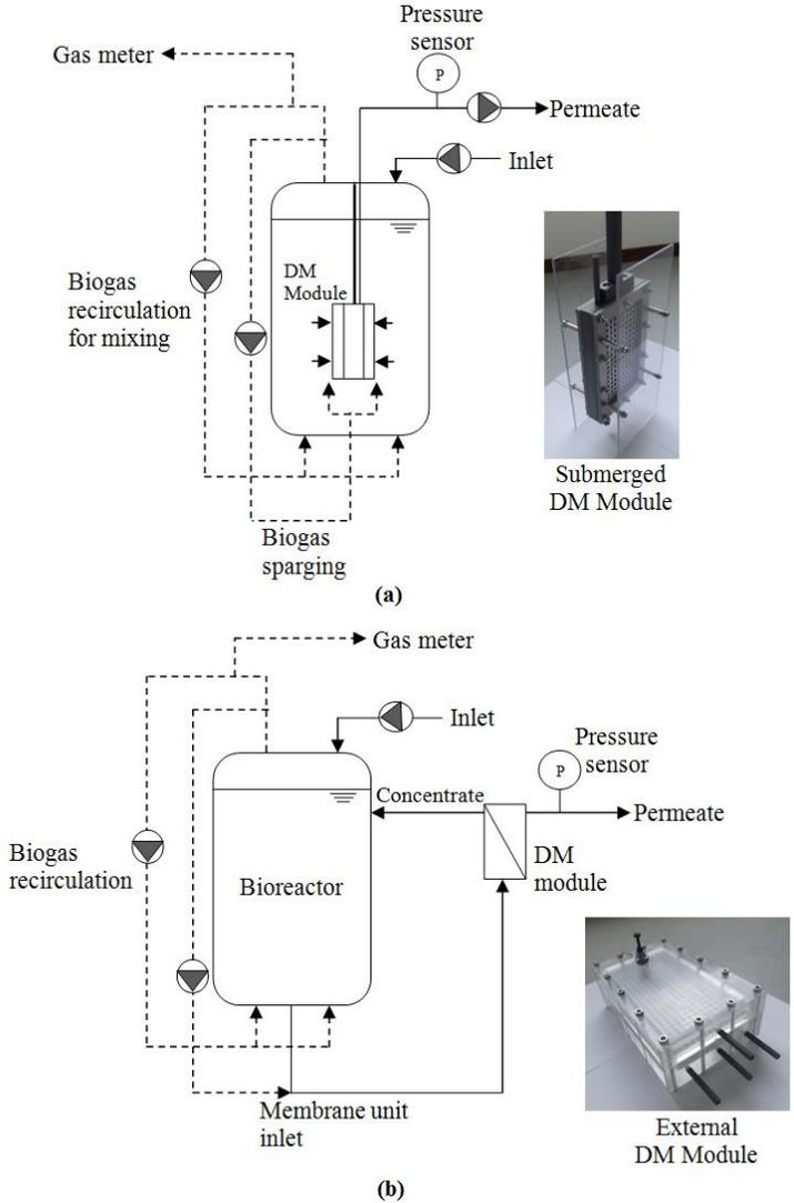
**Figure 6.1.** Laboratory scale set-ups: (a) submerged AnDMBR, (b) external AnDMBR.
