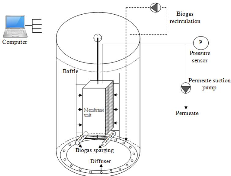
**Figure 3.1.** Submerged AnDMBR set-up.
