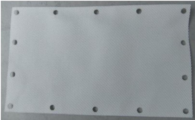
**Figure 4.3.** Mono-monofilament filter cloth.
