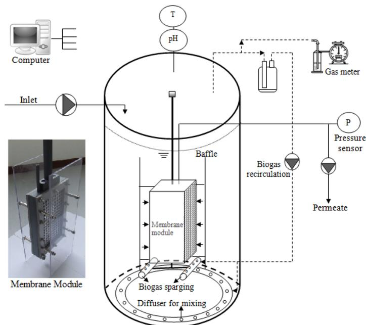
**Figure 4.1.** Schematic diagram of the submerged AnDMBR set-up.
