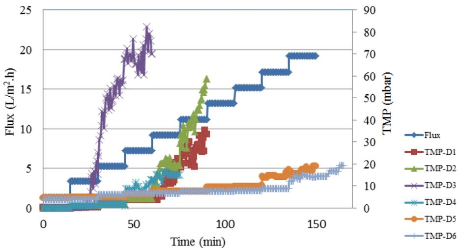
**Figure 3.3.** Critical flux determination for different support materials.
