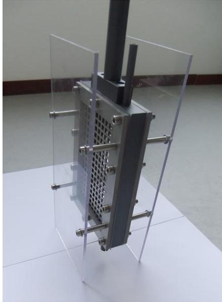
**Figure 4.2.** Submerged membrane module with two baffles.
