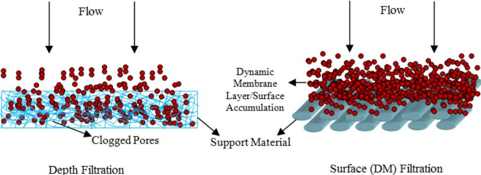
**Figure 3.10.** Difference between depth and surface filtration.
