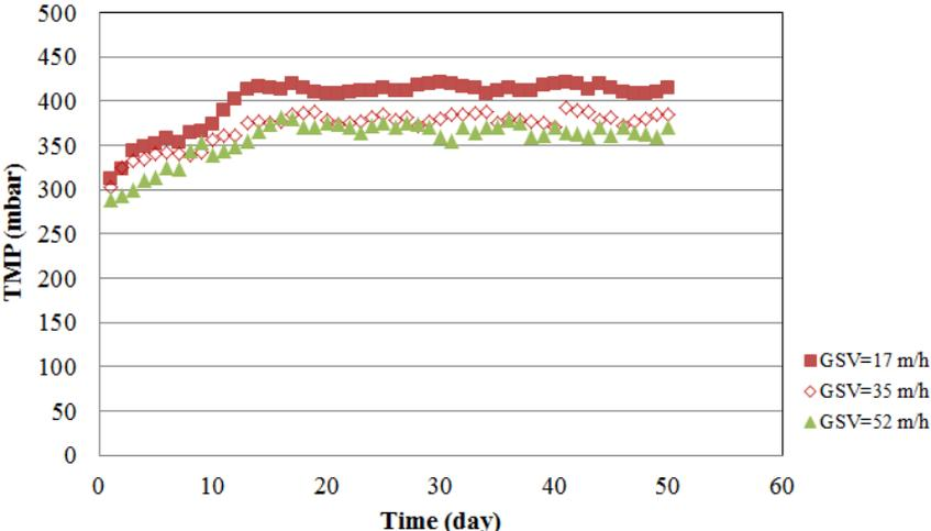
Figure 7.3. TMP at different GSVs.
