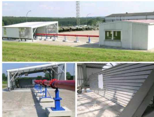
Figure 3.2: Images of the pressurised air cannon at IABG in Lichtenau.
