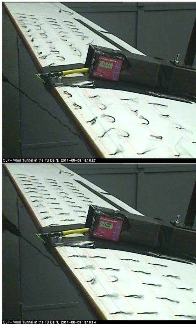
Figure 1.3: Example of flow separation control with the NS-DBD plasma actuators on a large scale model. top — no actuation, bottom — with actuation.
