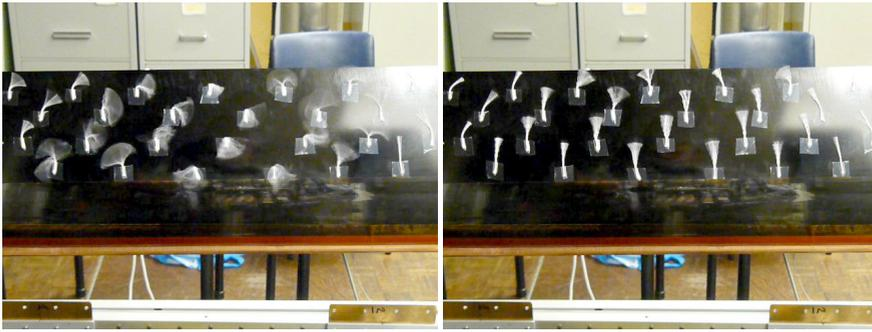
Figure 2.8: Separation elimination with NS-DBD plasma actuators. Left: actuation off; right: actuation on.
