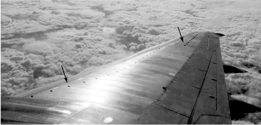
Figure 2.2: Rows of vane-type vortex generators (indicated by arrows) installed on a surface of an airliner wing.
