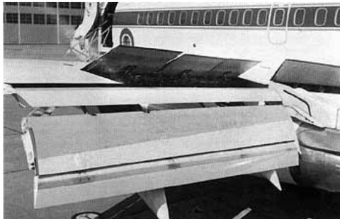
Figure 1.2: Example of elaborate high lift devices: triple slotted flaps on a wing of Boeing-737 airliner. Image: NASA.
