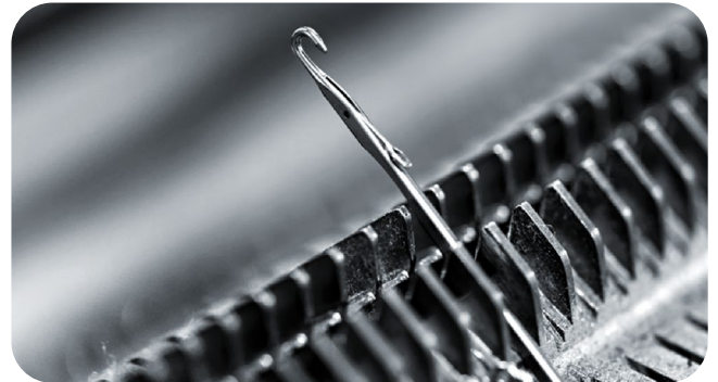
Figure 9, Close up of a machine needle in a flat bed knitting machine.
