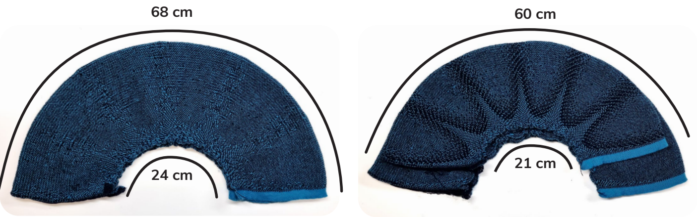
Figure 90, Gradient 1:4 (left) and 1:1 (right) sphere-like samples.
