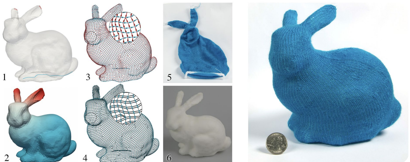
Figure 21, Automatically knitting the Stanford bunny. The system begins with an input mesh with user-specified starting and ending cycles (1) that are interpolated to define a knitting time function (2), remeshes the surface to create a row-column graph that represents the knit structure (3), traces the graph (4), and generates stitch instructions that are scheduled for machine knitting. The machine-knit skin (5) is a good fit for a foam replica of the input model (6). [63]
