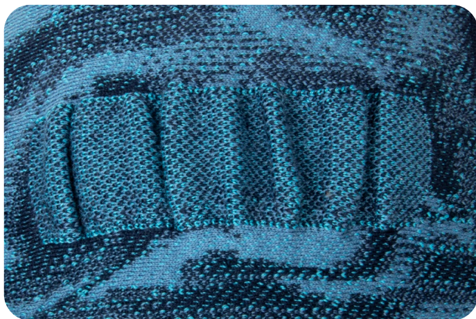
Figure 33, Swatch in preparation for the project with a different ratio of stitches and floats for the outer and inner sections, causing a surplus of material in the middle.
