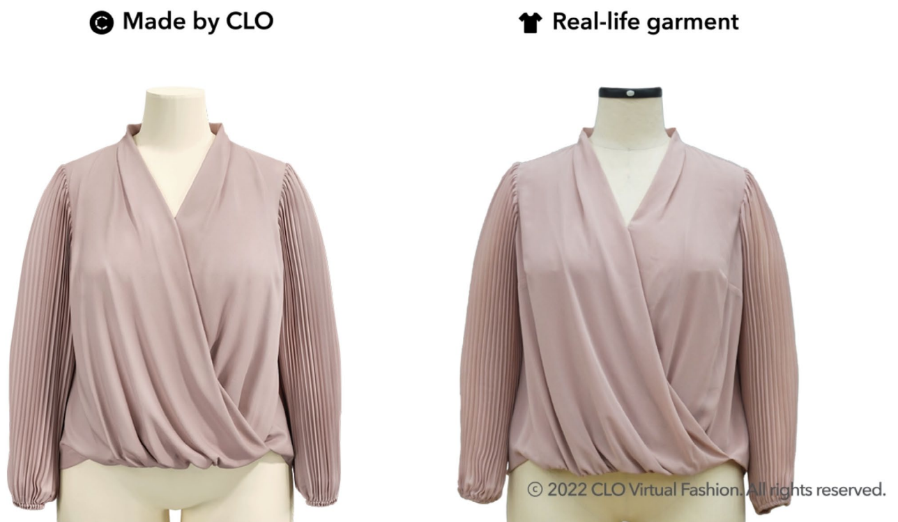
Figure 5, Comparison of a garment simulated in CLO3D and the real-life version [15].
