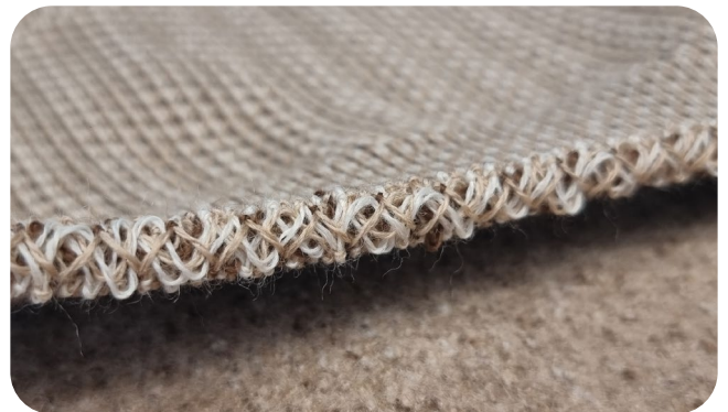
Figure 10, Cross section of a double-layered knitted fabric.
