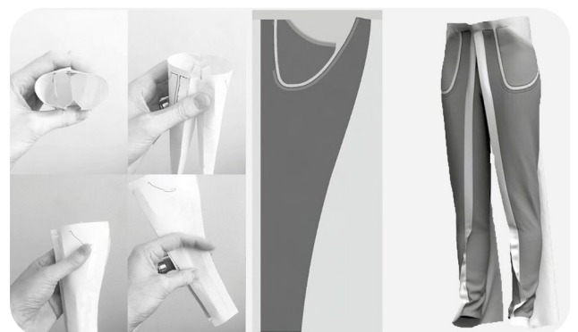
Figure 17, 3D woven pants where the legs and pockets are woven into the fabric in different layers. [57]
