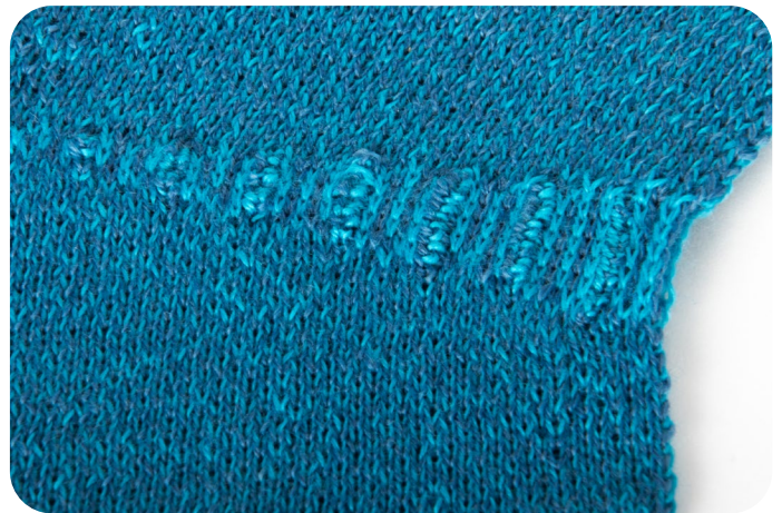
Figure 51, Close up of sample SL_1, which has visible and tactile ridges in the material.
