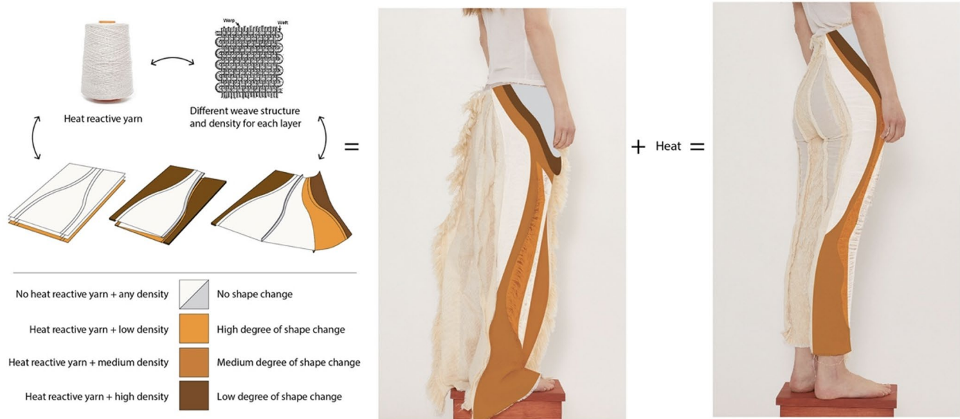
Figure 18, Yarn, weave structures, and textile-form construction work in symbiosis to produce specific shape change behaviours. [8]
