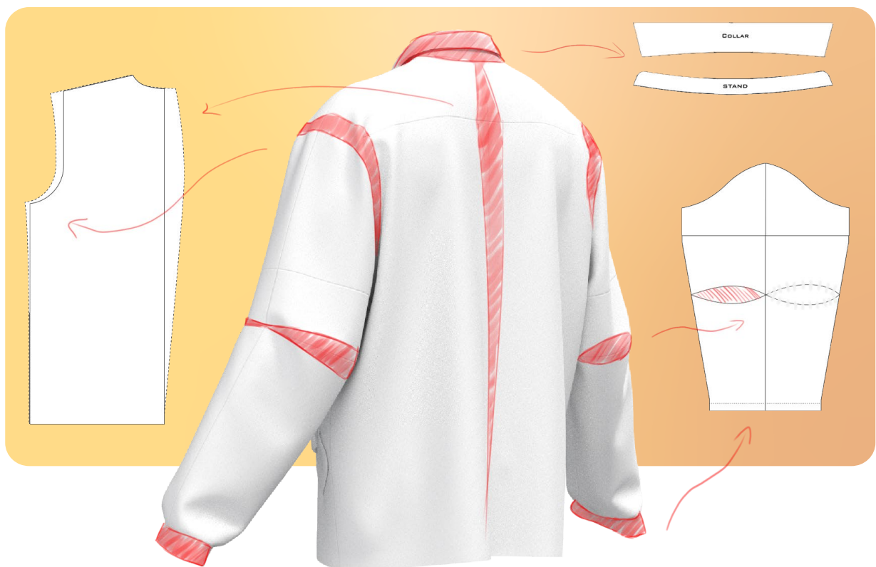
Figure 61, Each designed segment with the intended pattern shape, based on the desired shape changes.
