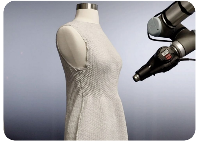
Figure 19, 4D Knitted dress by MIT shrinks around a body to create a personalised fit, using a robotised heat application process. [79]
