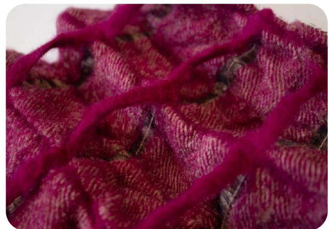
Figure 20, Woven sample with multiple layers and seperated long floats that shrink more, creating a 3D textured fabric. [4]
