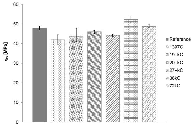
Figure 9: Absolute ILSS values for heated GLARE 5-2/1-0.3 specimens HGL1 to HGL6 thermal cycled between -20 and 80 °C (cf. Table 1).
