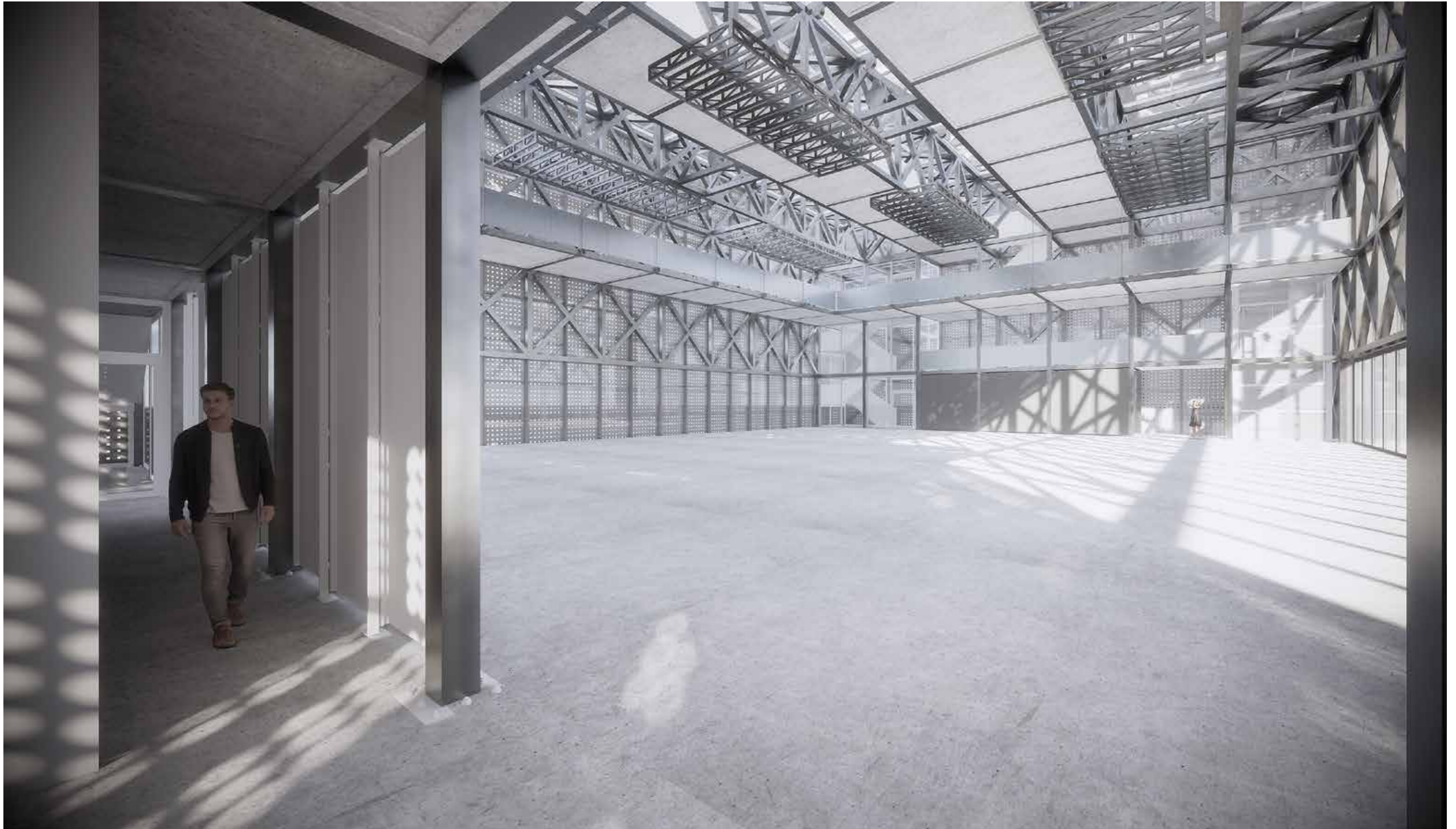
Visualisation showing the effect of the perforated aluminium facade plates on daylight entering inside the building. Seen from the main event space at +2.
