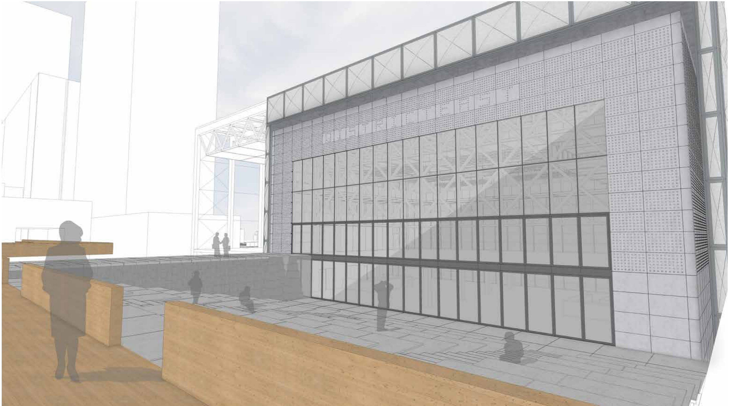
Visualisation showing the effect of the perforated aluminium facade plates.
