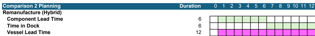
Figure 6.4: Vessel Lead Time, Component Lead Time and Time in Dock Shown in Planning for Comparison 2
