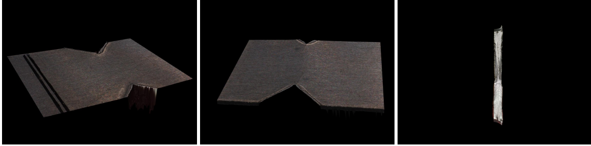
Figure 5.29: Specimen C2-01 – optical scans of the notch-root region at three stages: (left) Stage 1, pre-test; (centre) Stage 3, at the point of interruption; (right) Stage 4, the fracture surface after loading was resumed to failure. The right-hand panel views the fully separated fracture face edge-on, with the stable-growth region and the demarcated final-fracture zone both visible; the material surrounding it is intact beam, not an unbroken ligament. Panels are rendered with photographic surface texture rather than height colour-mapping, and are not to a common scale.
