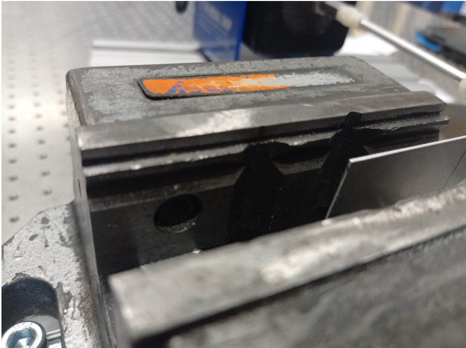
Figure 6.1: Clamping arrangement used for the Group C1 campaign, at the fixed end of the specimen. The jaw faces of the machine vice carry a stepped and grooved profile intended for gripping round or irregular stock, and scoring and edge damage from prior use are visible on the jaw surfaces.
