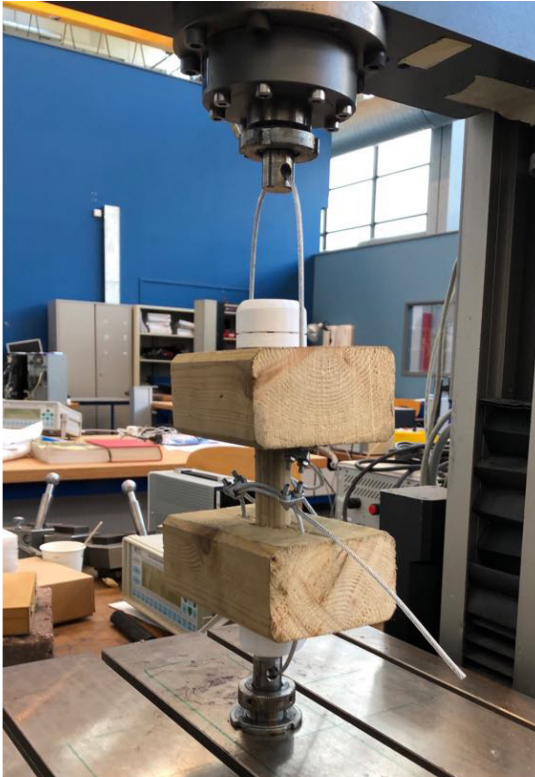
Figure 4.33 Tensile strength test 3D printed connector s
