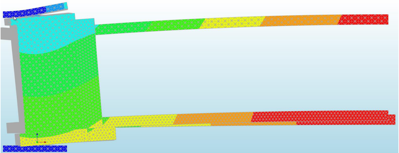
FIGURE 54 THE BOTTOM PIN IS STARTING TO DEFORM AND SINCE THERE ARE TWO ANCHORS THERE THE DEFORMATION SHOULD BE LOWER AT THE BOTTOM
