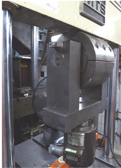
Figure 8: Hydro-bush dynamic testing at 100KN servo-hydraulic test bench
