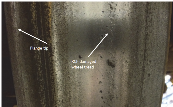
Figure 23: Wheel tread with RCF crack damage
