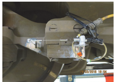
Figure 6: Detail - instrumented radial arm (measuring displacement)
