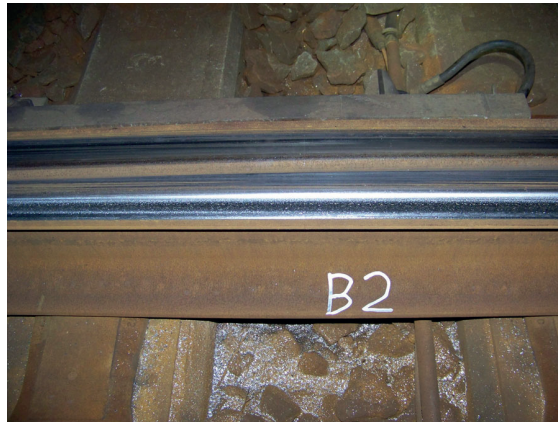
Figure 14. Switch panel of ‘severely’ wearing switch (left switch and stock rail). Wear debris present, high roughness of gauge face. No lubrication marks.
