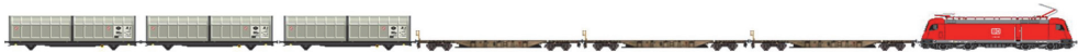
Figure 10: TAC established on the basis of vehicle type, speed and for freight wagon the individual load. For example: loco class x – 80 km/h, three wagons class y -full, three wagons class z-empty (source: SBB).
