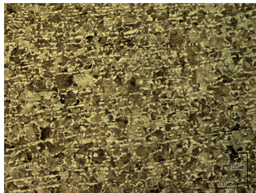
Fig. 9. Microstructure at area ‘W’(transverse cross section). The rail web material shows a texture composed of pearlite (brown) and lines of free ferrite (white). (For interpretation of the references to colour in this figure legend, the reader is referred to the Web version of this article.)
