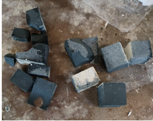
Figure 55: Prism samples after 28 days, showing severe cracking.
