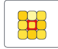
Figure 11: Central pixel (highlighted red) is detected. Then the hue value of this pixel and all its neighbours are averaged to reach an approximate hue value.
