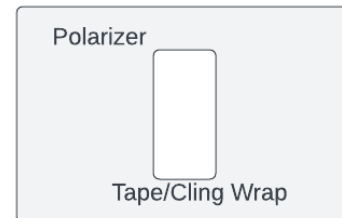
Figure 13: Pattern chosen for all experiments - a single rectangular strip of the material.
