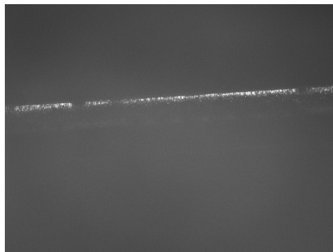
Figure 3.4: Image of a resonator in the LDV set-up of Figure 3.3 . The part of the beam that shows reflection, generally produces the best signal, resulting in sufficient back scattered light to detect a frequency shift.
