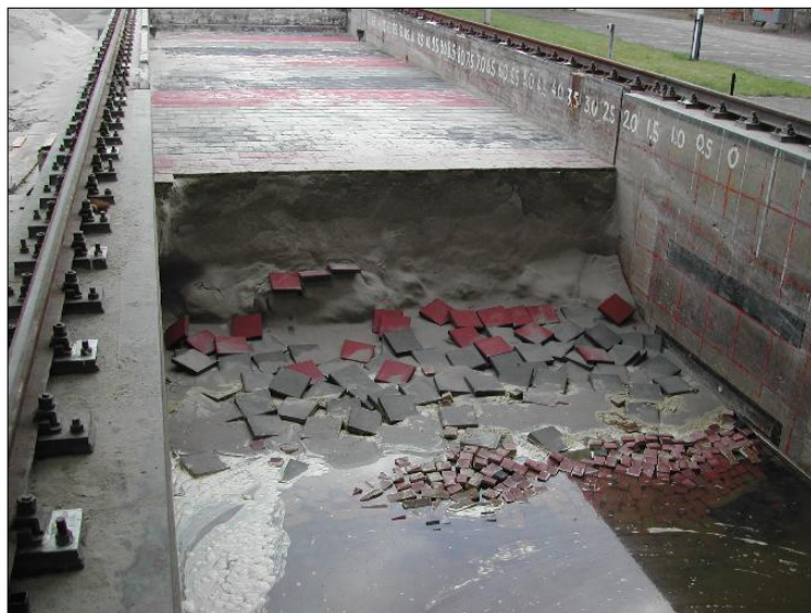
b. Dune and revetment after Test T11D
