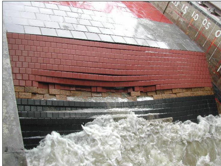
a. Wave attack during Test T11C
