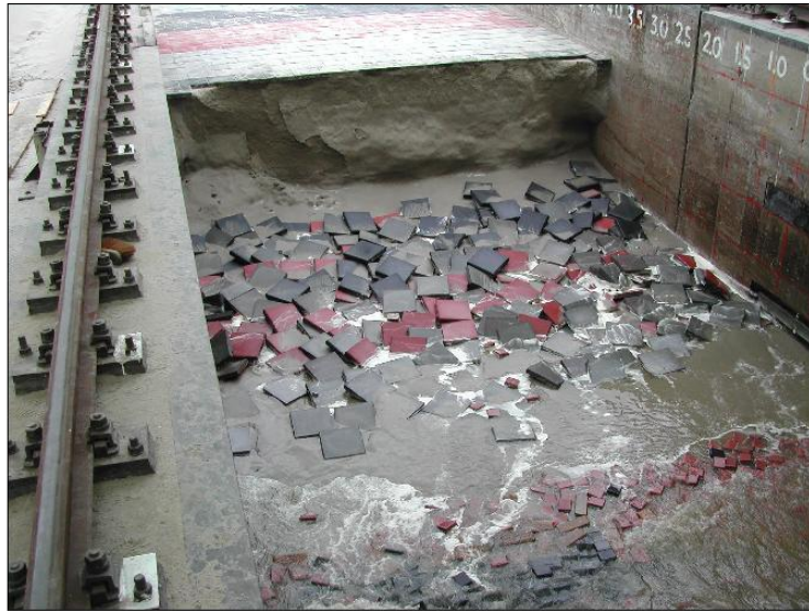
a. Dune and revetment after Test T11E
