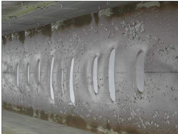
b. Holes in bed profile around 75 m from wave board
