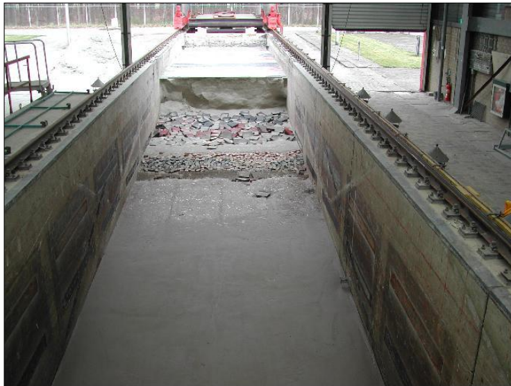
b. Dune and revetment after Test T11E in dry flume
