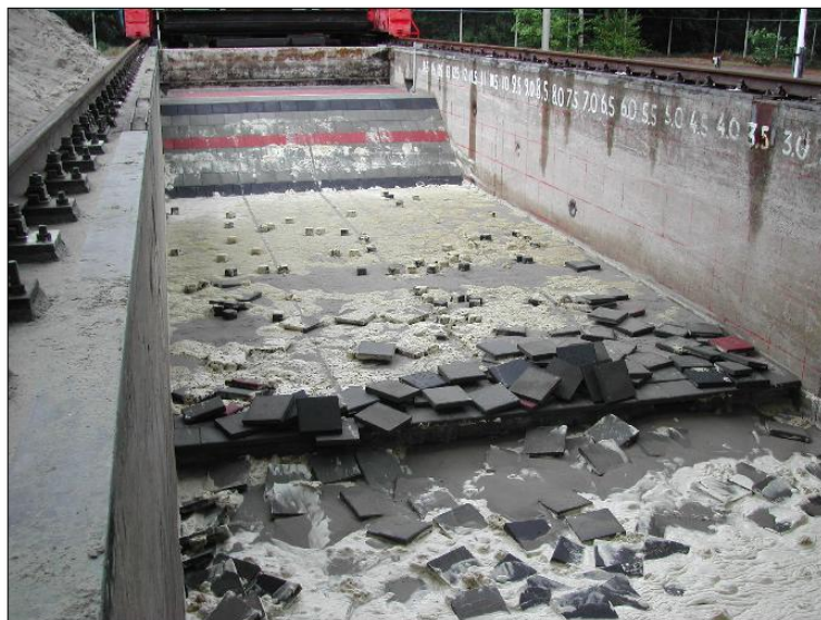
b. Dune and revetment after Test T13B
