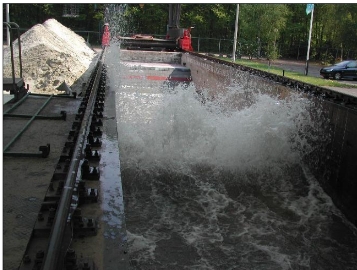
b. Wave impact at vertical part of revetment
