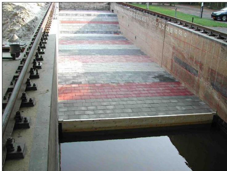
b. Revetment before Test T12
