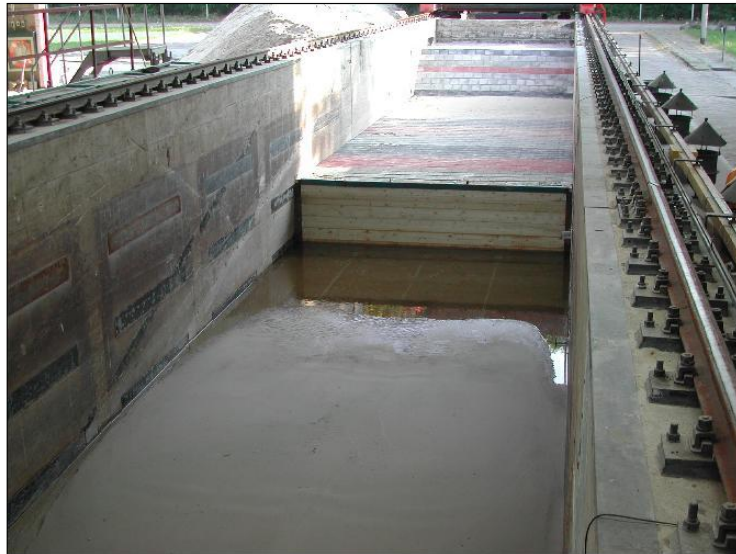
a. Dune and revetment after Test T12
