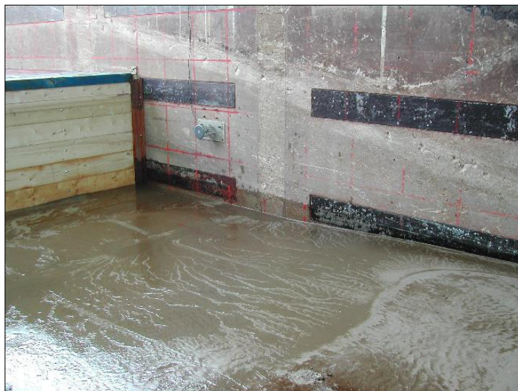
b. Scour hole after Test T12 in dry flume
