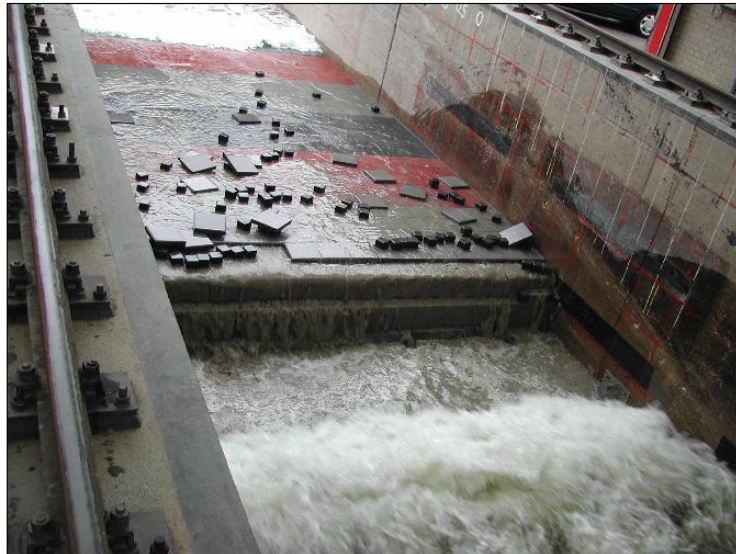
a. Dune and revetment during Test T13A
