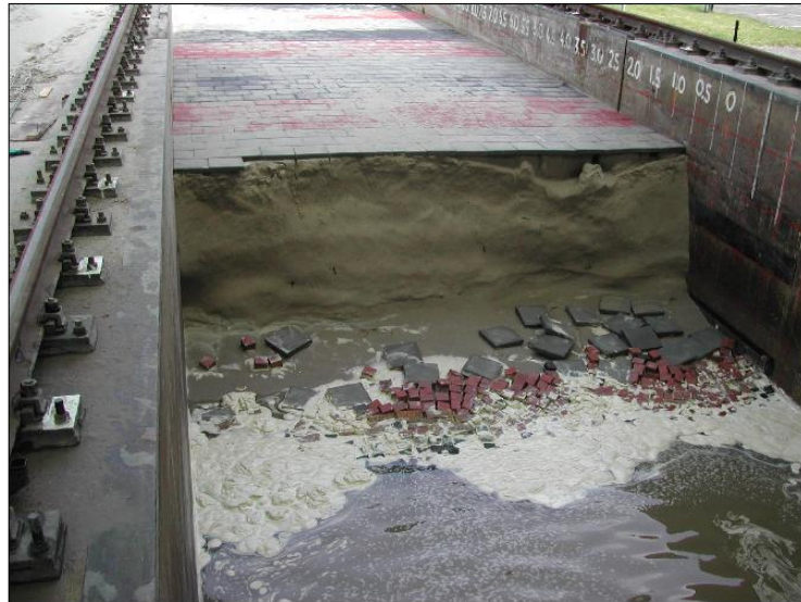
a. Dune and revetment after Test T11C
