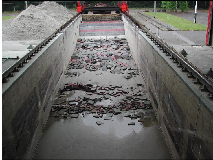
a. Dune and revetment after Test T13 in dry flume
