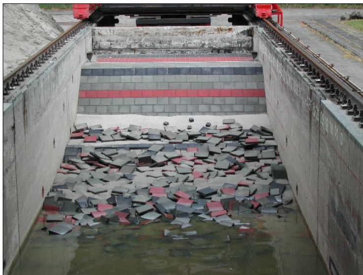
b. Dune and revetment after Test T13E
