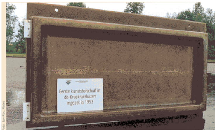
Figure 7.1: Composite steel slide in the Kreekraksluizen (1993-1997). (Honselaar, 1999, page 9)
