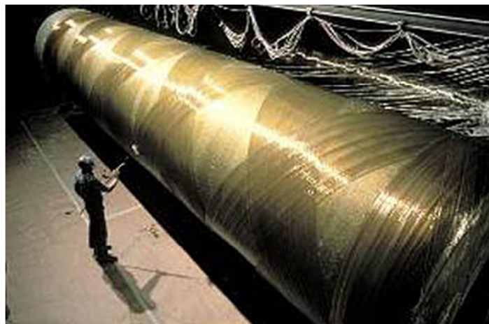
Figure 3.25: FRP pipe production, by filament winding (Fibrex)
