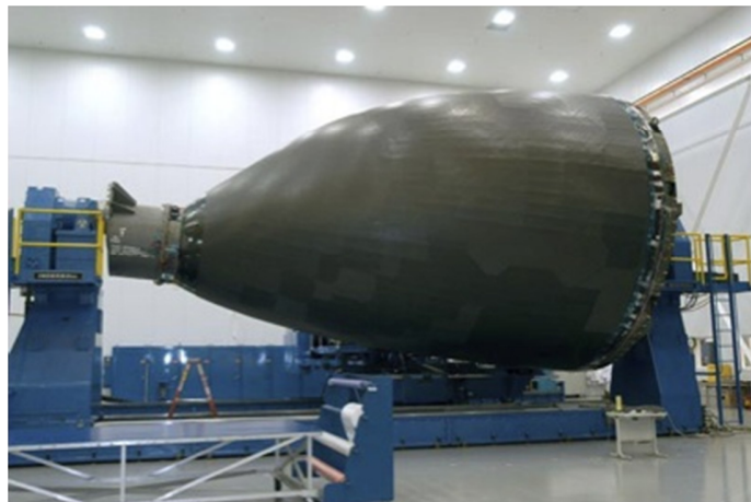
Figure 3.3: Filament Wound Boeing 787 Fuselage (Groh, 2012)
