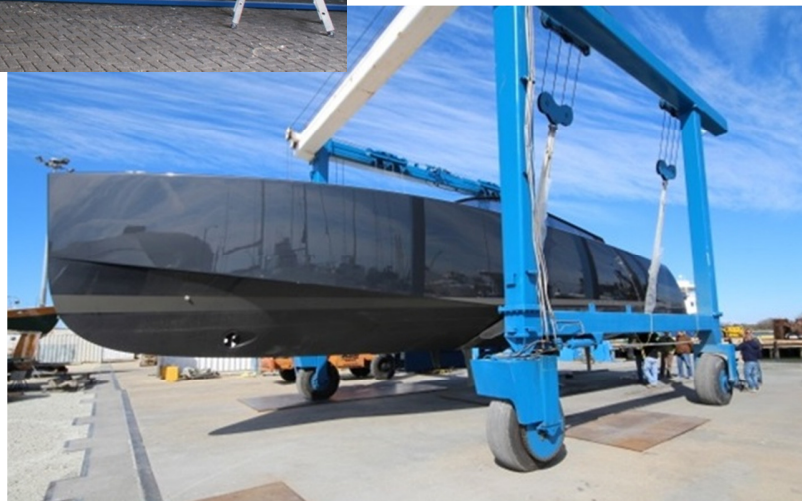
Figure 3.6 & 3.7: Van Dutch project, yacht build out of FRP composites ( Nedcam )
