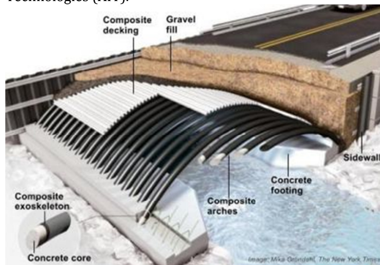
Figure 3.9 (above): Illustration of the ‘Bridge-in-a-Backpack’ system. (AIT)
