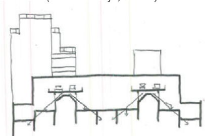
In the attic two conveyor cover the length of the building and distribute the grain.
