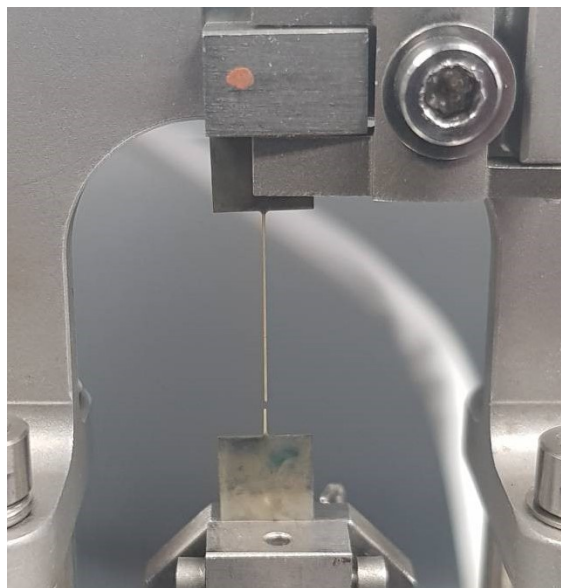
Figure 3.6: Failed tensile test specimen.
