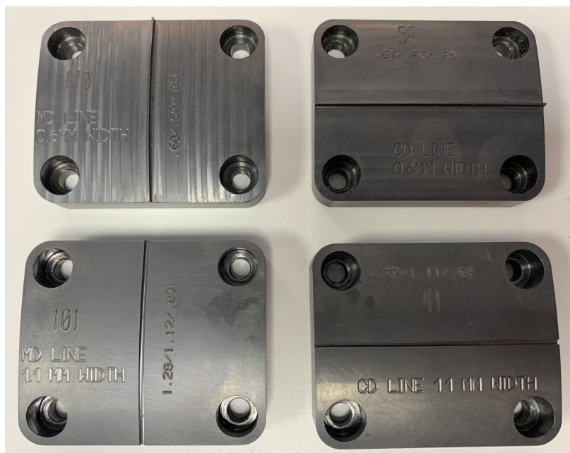
Figure 4.3: Four die segments: The top row shows male dies and on the bottom row shows female dies. The left male and female dies form web channels. The right male and female dies form cross-web channels.
