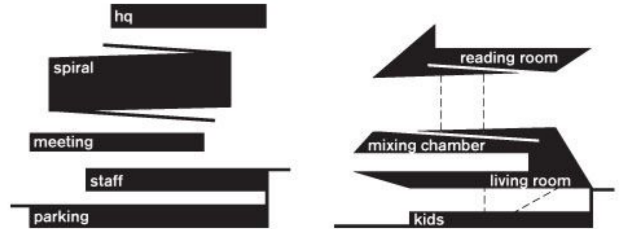
Seattle library, OMA, 2004, the division demonstrated in section between dedicated and fluctuating spaces.
