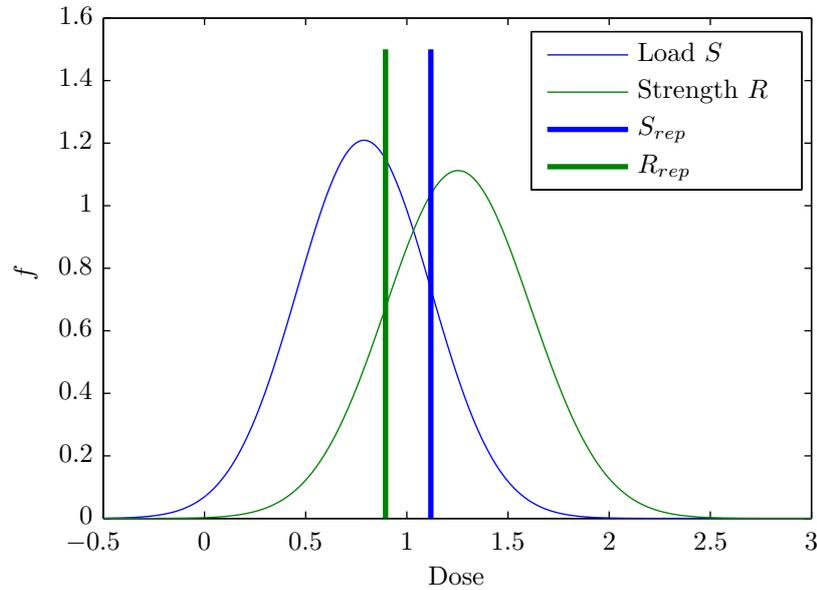
Figure 4.2: Figure 4.1 is expanded with deterministic values for strength  $R_{rep}$  and load  $S_{rep}$ . The values are located at a distance of one standard deviation from their respective means, which would lead to failure
