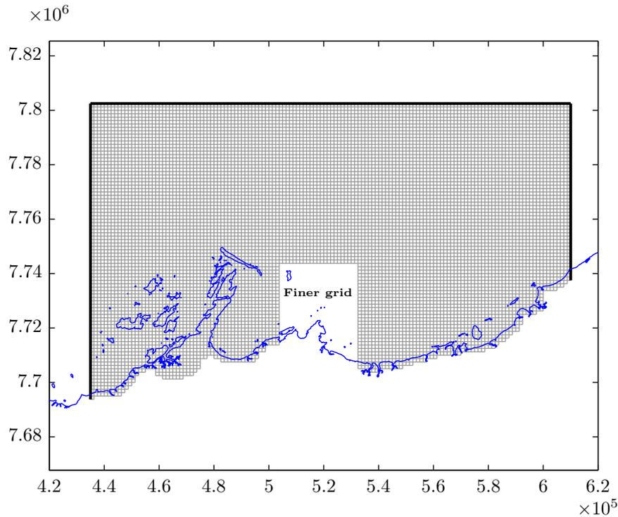
Figure 5.1: The region of interest with rectilinear grid. The grid sizes are 1250  $m$  by 1250  $m$ . The dredging area and the area around it are covered with a finer grid. The Domain Decomposition toolbox within DelftDashboard allows for this grid refinement.
