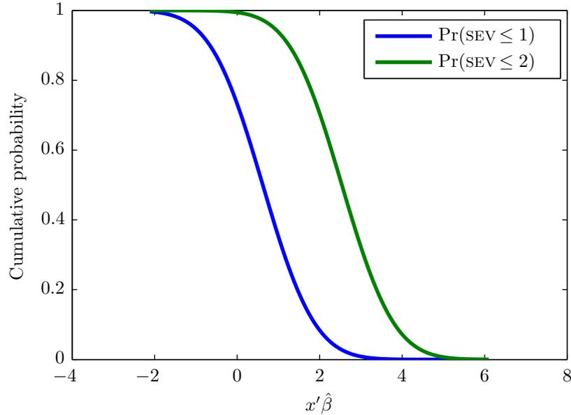
Figure 2.3: Dose-response curves. An ordered probit model is fitted using Maximum Likelihood. The cumulative probabilities  $\Pr(\text{SEV} \leq j)$  are plotted as a function of  $x'\hat{\beta}$ , where  $x_1 = \log(C)$ ,  $x_2 = \log(T)$  and  $\hat{\beta}$  as specified in Table 2.2. The probability  $\Pr(\text{SEV} \leq 3)$  is 1 for every value of  $x'\hat{\beta}$
