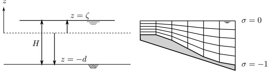
Figure B.1: Frame of reference (left) and  $\sigma$ -grid (right)
