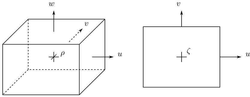
Figure B.3: Grid staggering, 3D view (left) and top view (right)
