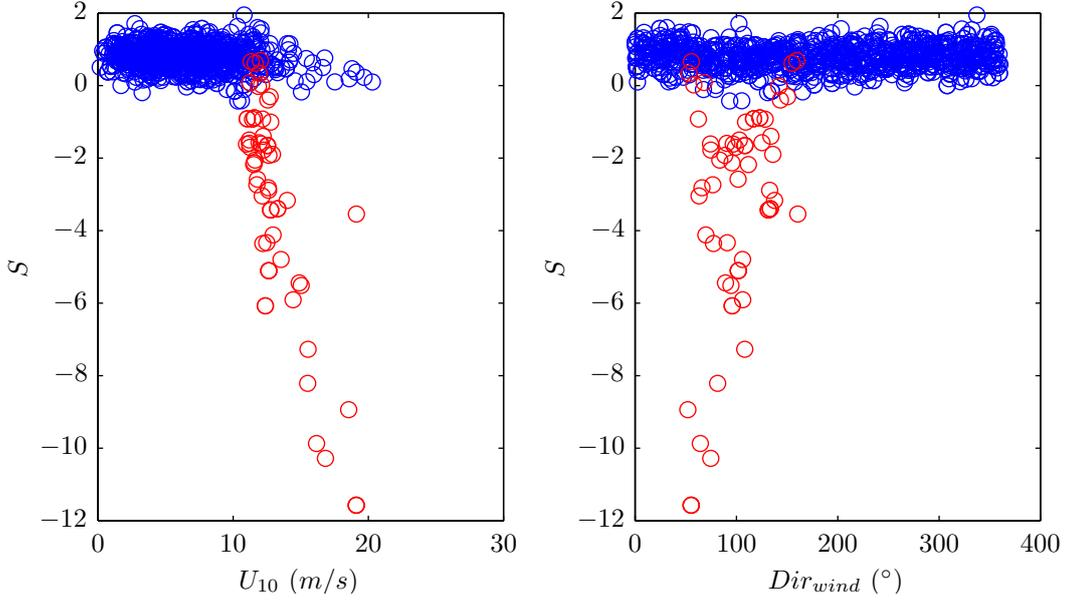
Figure 5.3: Scatter plot with load  $S = (x'\hat{\beta})_{crit}$  as a function of wind velocity  $U_{10}$  (left) and wind direction  $Dir_{wind}$  (right) for sensitive receiver  $SR2$ . The red circles meet the criteria  $U_{10} > 10.95 \text{ m/s}$  and  $50^\circ < Dir_{wind} < 161^\circ$  and are excluded from further analysis. However, they remain important simulation results.
