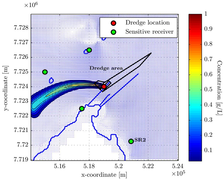
Figure 3.1: Plume dispersion after one hour of dredging. The sensitive receiver *SR2* is located South-East of the dredging project.
