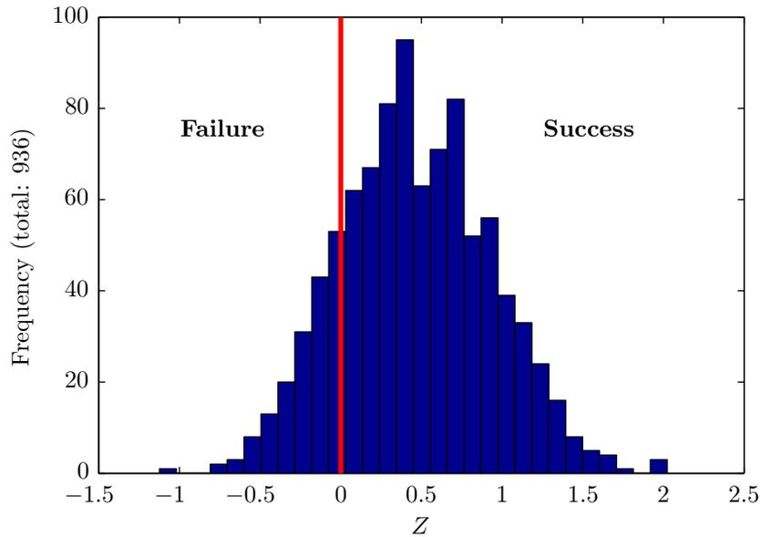
Figure 5.5: Histogram of  $Z$ -values after a Monte Carlo simulation.  $Z < 0$  equals failure, according to Equation 4.6. The result of the simulation is  $784 + 64 = 848$  successes and 152 failures, which leads to the conclusion that the failure probability  $\Pr_f = 15\%$ .
