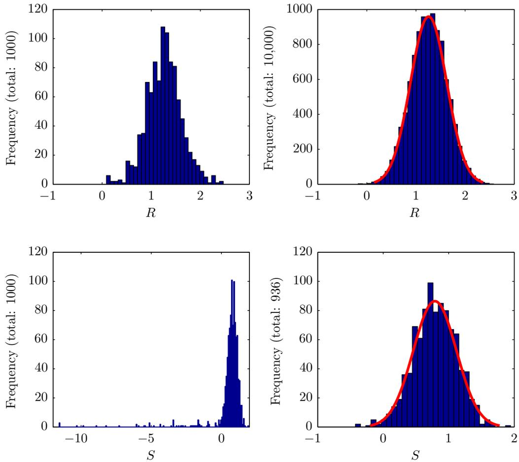
Figure 5.4: Histogram of values for strength  $R$  (top) and load  $S$  (bottom) after a Monte Carlo simulation. The number of strength realizations is increased to 10000 (top right) to confirm a normal population distribution. The simulation results that meet the criteria  $U_{10} > 10.95 \text{ m/s}$  and  $50^\circ < Dir_{wind} < 161^\circ$  are included (bottom left) or excluded (bottom right) to allow a normal distribution fit.
