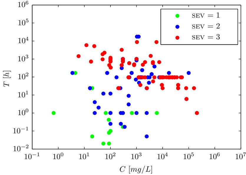
Figure 2.2: Scatter plot on a log-log scale with severity of ill effect (SEV) as a function of suspended sediment concentration  $C$  and exposure duration  $T$ . SEV = 1 leads to behavioral effects, SEV = 2 to sublethal effects and SEV = 3 to lethal and para-lethal effects
