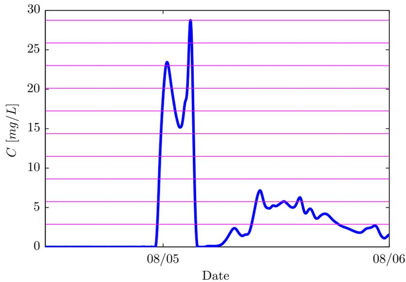
Figure 3.2: Time series of suspended sediment concentration  $C$  for sensitive receiver *SR2*, located as specified in Figure 3.1. The maximum level is divided into 10 equal parts, which enables determination of exceedance durations.
