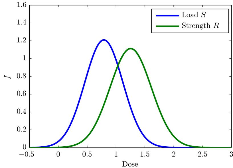
Figure 4.1: Probability density function of the load  $S$  and the strength  $R$  after a Monte Carlo simulation with sample size a thousand. The development of these particular curves will be explained in [Chapter 5](#)
