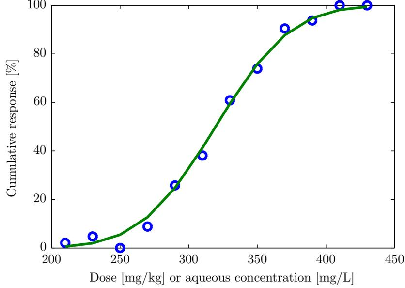
Figure 2.1: Manually fitted cumulative dose-response curve, which is the result of a lethality experiment. Data points are indicated as circles. The curve can be interpreted as the empirical distribution function of the resistance of the sensitive receiver.
