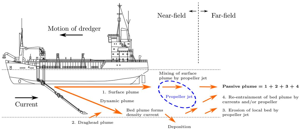
Figure A.1: Sources of a dredge plume near a TSHD (Spearman et al., 2011)
