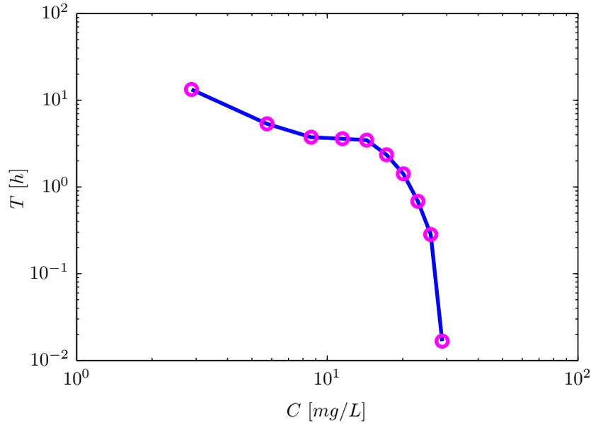
Figure 3.3: Load curve for sensitive receiver *SR2* on a log-log scale, as derived from Figure 3.2. The curve is the result of one simulation. It depicts the suspended sediment concentration  $C$  (on the x-axis) and the exposure duration  $T$  (on the y-axis) for which it is exceeded.
