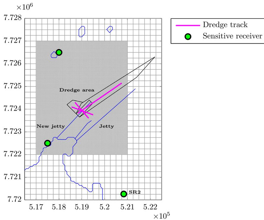
Figure 5.2: The dredging area with coarse grid (250 m by 250 m) and fine grid (50 m by 50 m). The dredge tracks cover approach channel, turning basin and berth pockets. The sensitive receiver *SR2*, which will be investigated, is located South-East of the dredging project.
