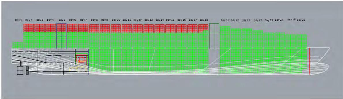
**Figure G.1:** Container arrangement; red = empty (2 ton), green = full (9 ton)
