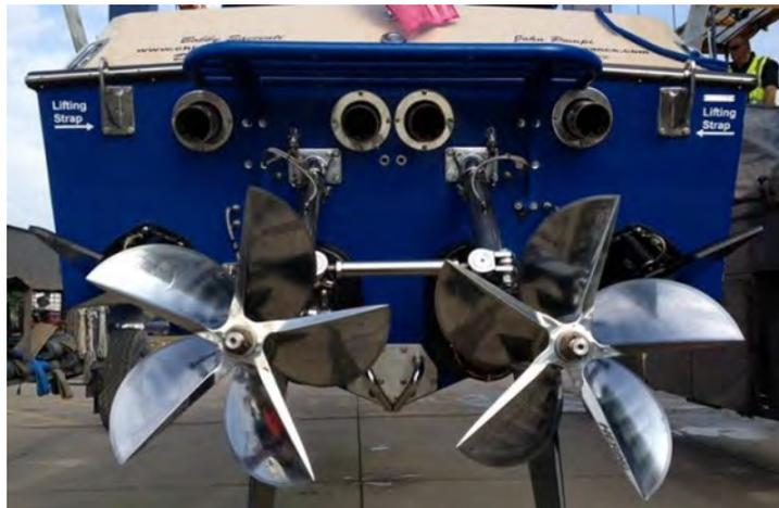
Figure 4.9: High speed propeller layout [168]
