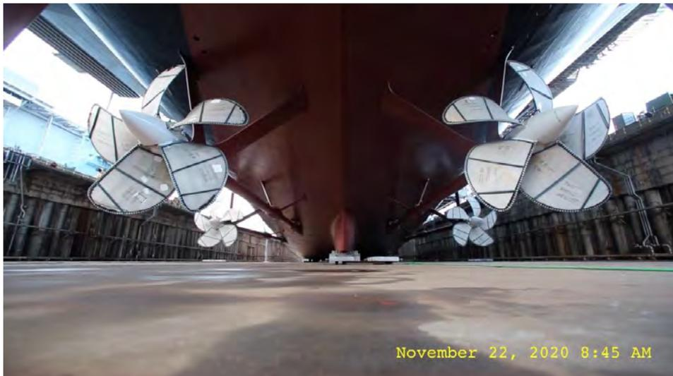
**Figure 4.3:** USS Gerald Ford propulsor layout [111]
