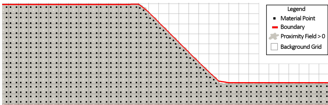
Figure 5.14: Initial condition of a slope stability problem used to address the problems regarding proximity field holes and boundary roughness. A visualisation of the proximity field larger > 0 is included.
