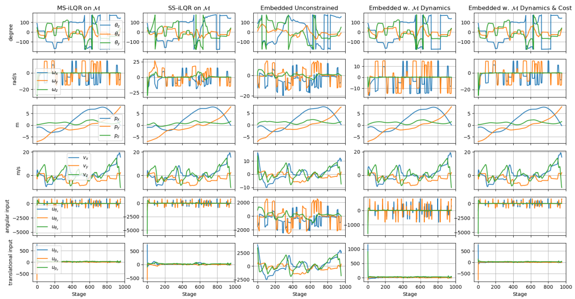
Figure 4-11: State and input for tracking on SE(3) with drone racing reference.
