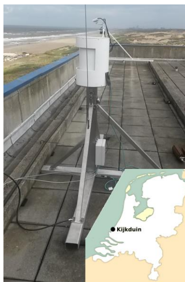
Figure 1: Experimental set up: A Riegl VZ2000 laser scanner is mounted on a steel frame on the roof of a hotel near the beach in Kijkduin, NL. The scanner is covered with a protective casing to shield it from wind and rain while not operating.
