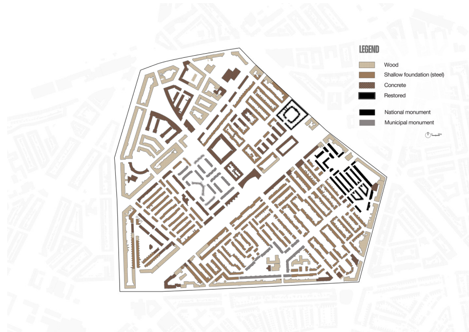
Figure 7: Foundations (TU Delft, 2025).
