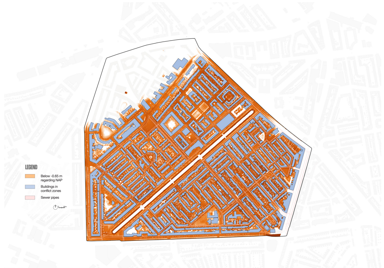
Figure 15: Zones below desired surface level (TU Delft, 2025).
