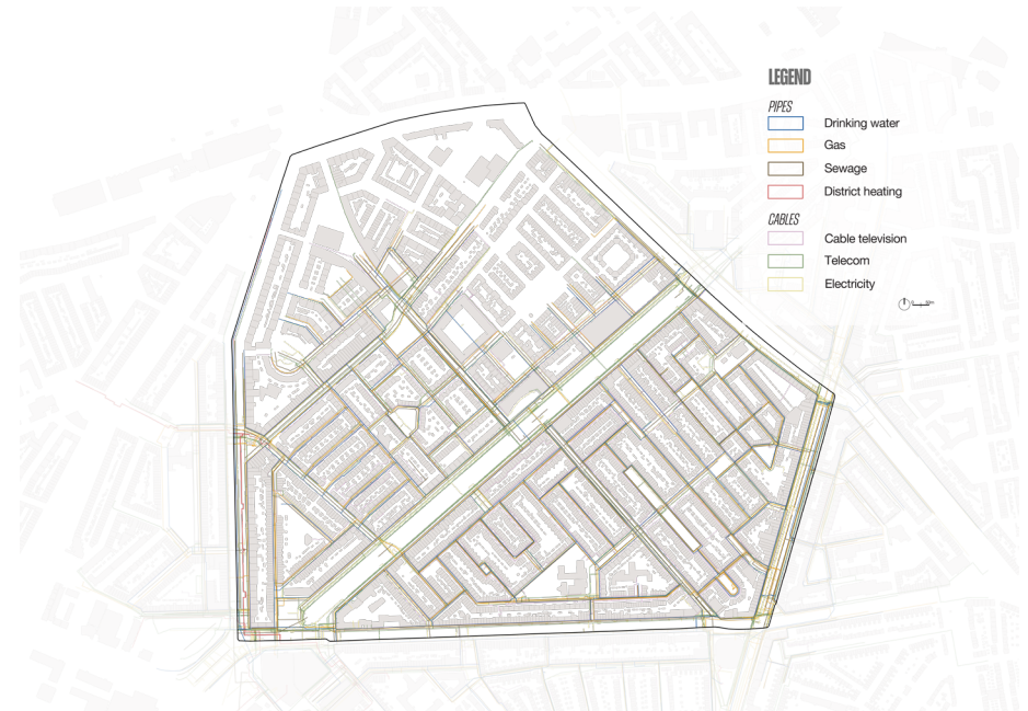
Figure 10: Cables and pipelines (TU Delft, 2025).
