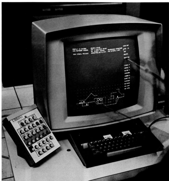
Fig. 17 URBAN5 workstation setup, pointing on the screen with a lightpen. (MIT Technology Review, c. 1969)
