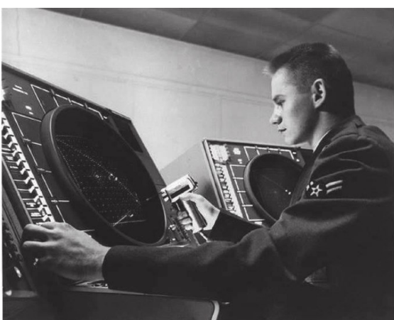
Fig. 2 The operator uses a lightgun and operates the console controls. (MIT Lincoln Laboratory, 1958)
