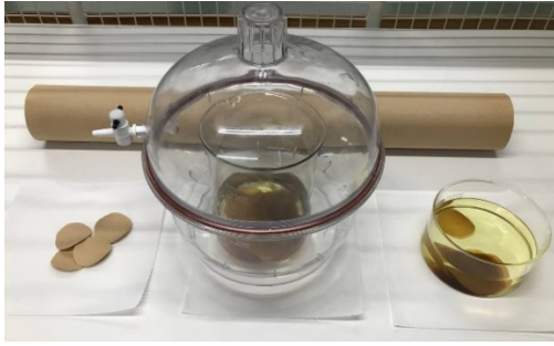
Fig. 1. Sample preparation. Paper roll, small circular paper samples, OIP samples stored inside a closed desiccator, OIP samples transferred to another glass container to be used for the test.
