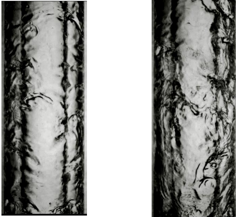
Figure 10: Experiments done at a U_{SL} = 1 \text{ cm/s} . The left graph is at a U_{SG} = 10.6 \text{ m/s} and the right one is at a U_{SG} = 8.5 \text{ m/s} which is close to the onset of liquid loading. The roughness and the chaotic nature of the liquid structures are more pronounced in the second case and therefore marks the start of churn flow.
