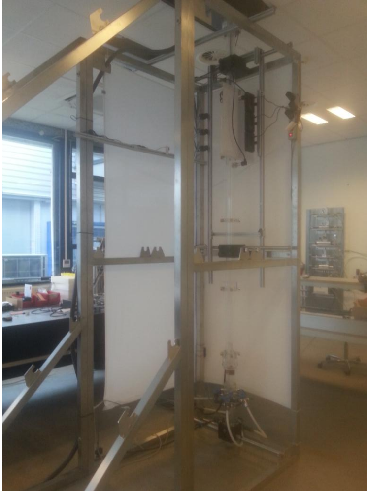
Figure 12: The experimental setup as built for the project. The equipment is designed to conduct tests with varying eccentricities, flow rates and even inclinations.
