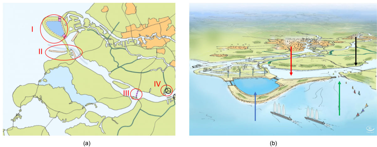
Figure 1.1: (a) Artist impression of what the Delta21 interventions would look like on the study domain (also see Figure 1.3): I - energy storage lake and pumps, II - new navigation channel and storm surge barrier, III - raised sill Haringvliet bridge, IV - new freshwater intake Strijensas. (b) Delta21 in bird's flight, left-to-right: energy storage lake, brackish tidal lake, Delta21 storm surge barrier and Haringvliet sluices. Source: Lavooij and Berke (2019)
