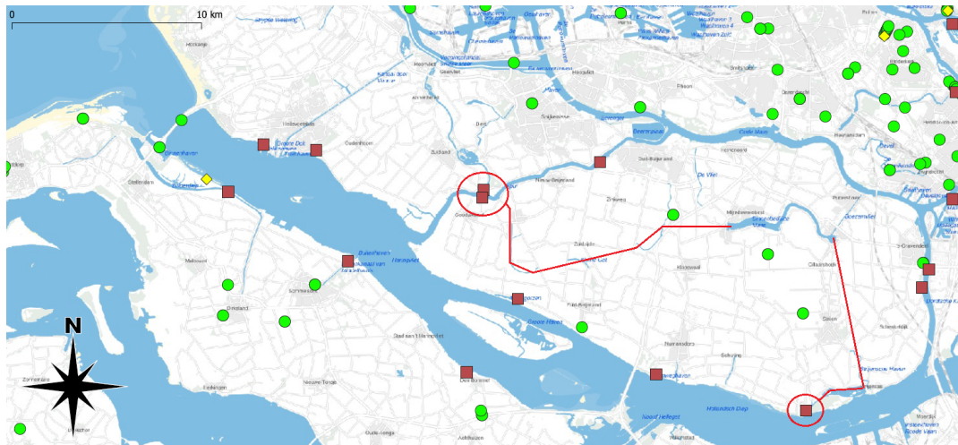
Figure 3.3: Drinking water intakes (yellow diamond), irrigation water intakes (brown square) and intakes for municipal water treatment (green circle) along the HV-HD. Relocation of Bernisse intake to the east indicated in red. Source: PDOK geodata.
