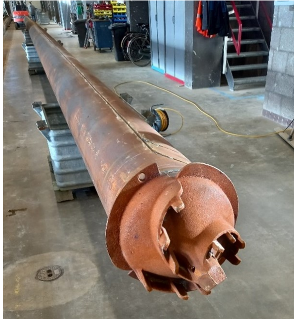
Fig. 2. The conical tip of a screw injection pile with a permanent casing ( Tubex pile)
