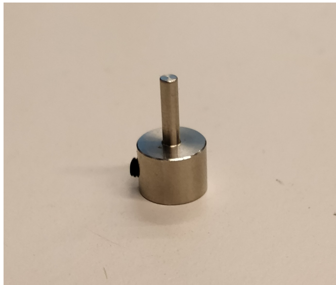
Figure C.5: A picture of the extension of the motor shaft used to find out the friction between the eccentric head and the drive bridge
