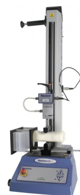
Figure 6.13: Mecmesin load tester used in the experiment
