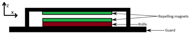
Figure 3.5: Pressure from top using magnetic repulsion
