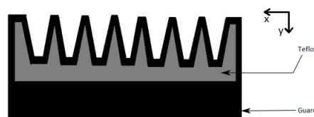
Figure 3.11: Friction reduced using embedded Teflon on the guard blade
