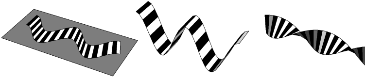
Figure 11. Ribbon geometry. The ribbon at left is planar and only modulated through geodesic curvature, the ribbon at center is only modulated through normal curvature, and the ribbon at right is purely twisted. A generic ribbon will have geodesic and normal curvature, as well as twist. Ribbons assume an ontological position between curves and surfaces.
