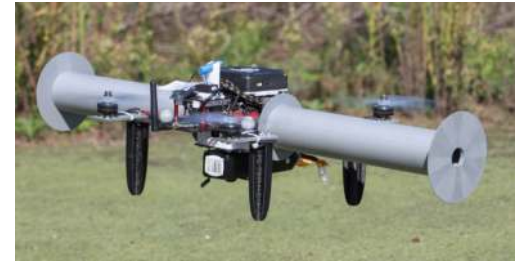
Magnus effect-based quadcopter system
