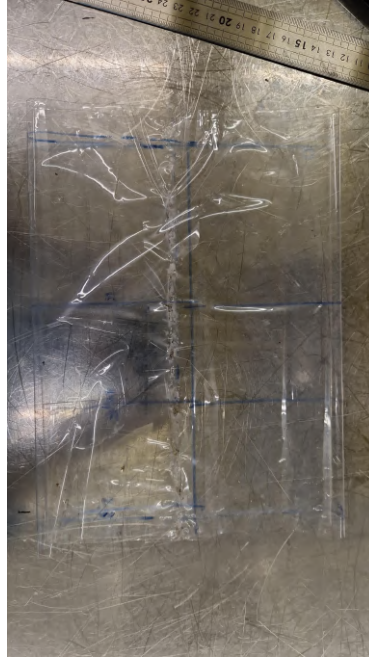
Figure B.5: Cylindrical bellow with completed melted seam.
