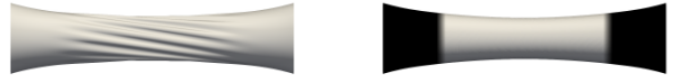
Figure 4: Stretched and twisted thin cylinder using Neo-Hookean material in isogeometric analysis [31]. Left figure shows the full Kirchhoff-Love shell model, while the right figure shows a wrinkle approximation based on tension-field theory. The black regions denote taut sections, while grey denotes a wrinkled region where a wrinkling model is defined based on Roddeman et al. [44]. While the shape of wrinkles is not calculated using the approximation, it should be noted that the general outline of the right structure is consistent with the left case.
