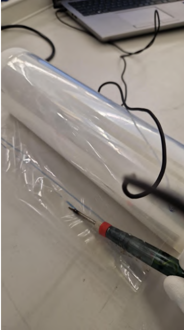
Figure B.4: Using a soldering iron to create a melted seam.
