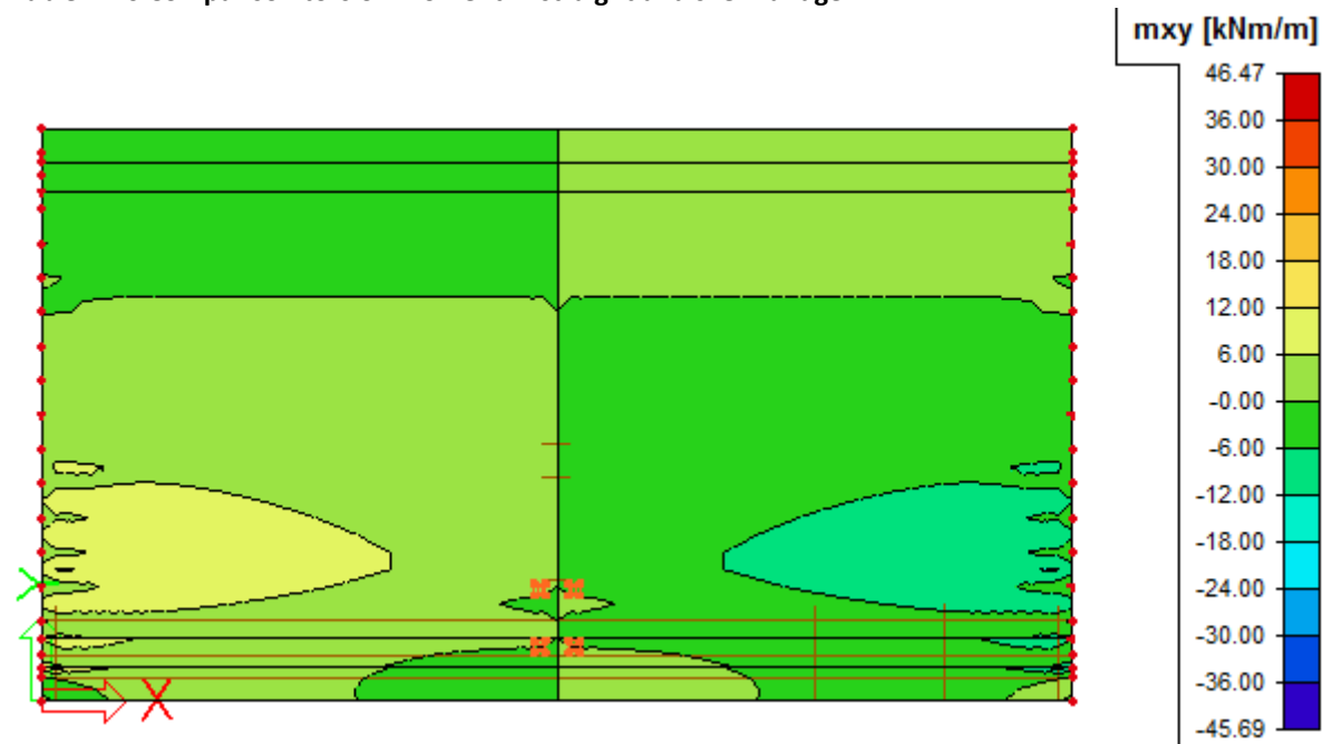
Figure B-15 Torsion in straight bridge due to load case 2
