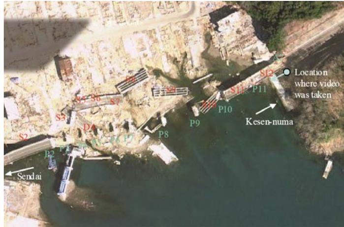
Figure 2- 12 Utatsu bridge situation after the Tohoku Tsunami (2011) [16].
