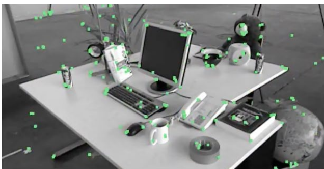
Fig. 2.5: Kudan 2018. SLAM Tracking, left: feature point detection, right: mapping these points and user location in 3D space
