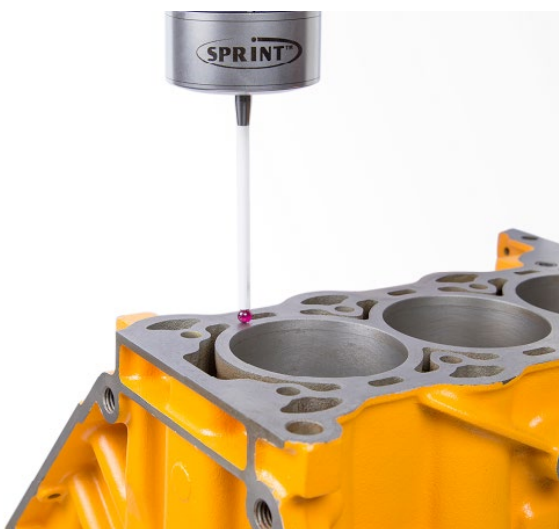
Fig. 2.8: Contact 3D scanning with a Sprint probe
