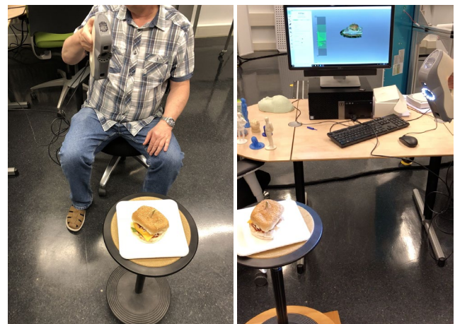
Fig. 4.1: Scanning the burger using the Artec Eva
