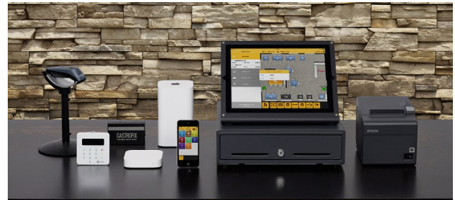
Fig. 2.37: The devices included in Gastrofix's POS system
