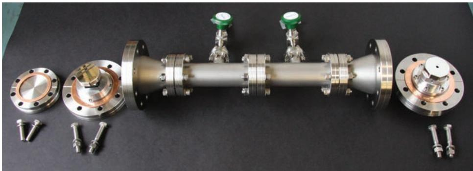
Figure A.1: Multipass cell components.
