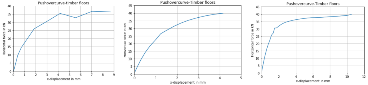
FIGURE 47: PUSHOVER CURVE 3D-MODEL-DOUBLE TIMBER FLOORS -DS, HJ, DIRECT LEFT TO RIGHT
