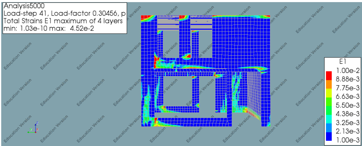
FIGURE 182: MAXIMUM PRINCIPAL STRAIN – STEP 41- SIDE-VIEW 2
