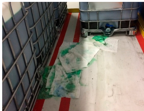
Figure 6. A cubitainer with leaking drain valves leading to a spill of the liquid content.
