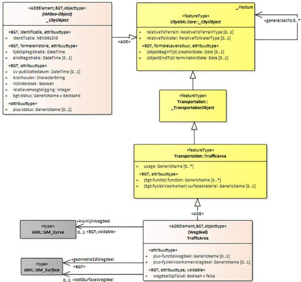
Figure 2.5: Example – IMGeo modelling of Wegdeel as subclass of CityGML-TrafficArea
