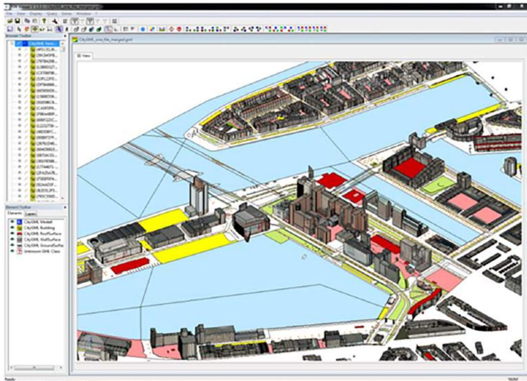
Figure 3.7: Visualisation of CityGML-IMGeo encoded data: CityGML LOD2
