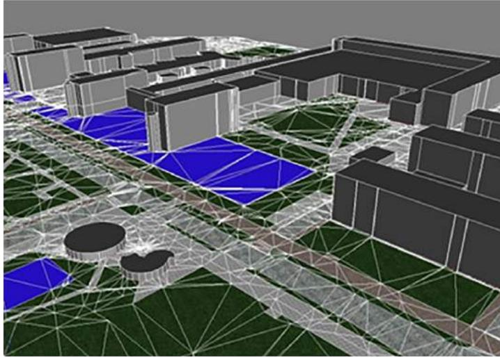
Figure 2.2: Triangulated terrain integrated with IMGeo objects (Emgard and Zlatanova, 2007)
