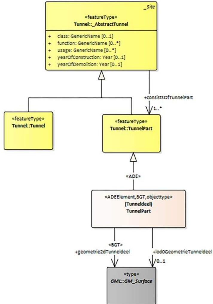
Figure 3.4: TunnelPart AD Element with 2D geometry
