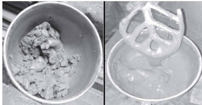
Figure 2: Workability of paste with FA-3 (left) and FA-4 (right)
