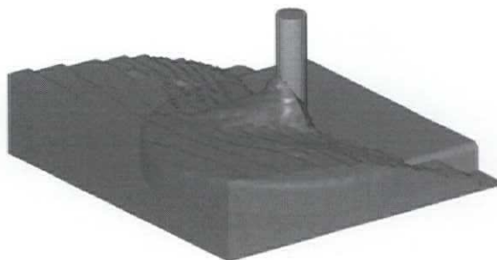
Figure 2.23: Snapshot of a simulation of green water flow on the deck of a fixed vessel
