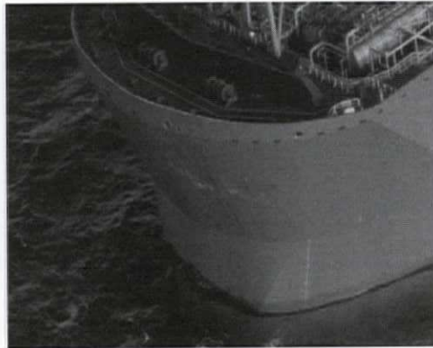
Figure 1.3: Wave impact damage causing dents to the bow of the Schiehallion FPSO
